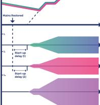
Dc voltage and AC current behaviour using the same value for delay time
